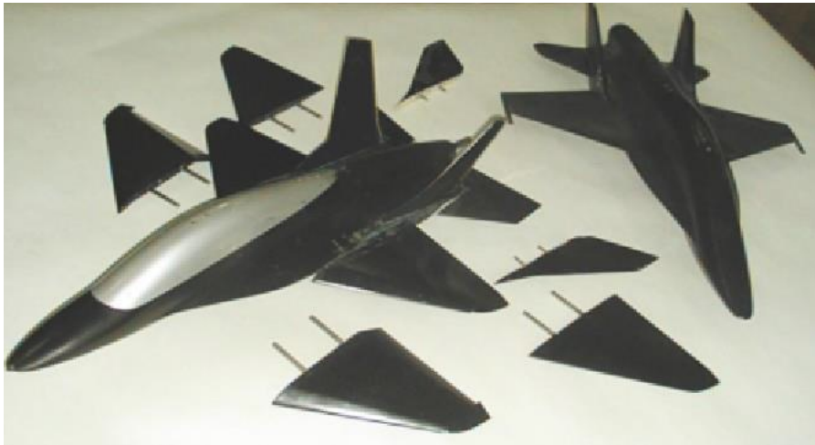
Fig. 5. Models used for testing in the wind tunnel [5]
