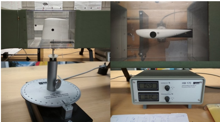
Fig. 5. The model is mounted in a workstation. Platform with a scale of attack angles and a device for reading the values of generated bearing and resistance forces
