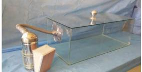
Fig. 1: The glass box and smoking machine. Hormonal assay:
