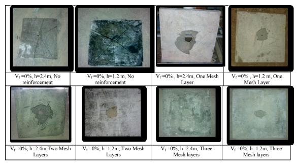
Fig. 7- The mode of failure of slabs under low velocity impact
