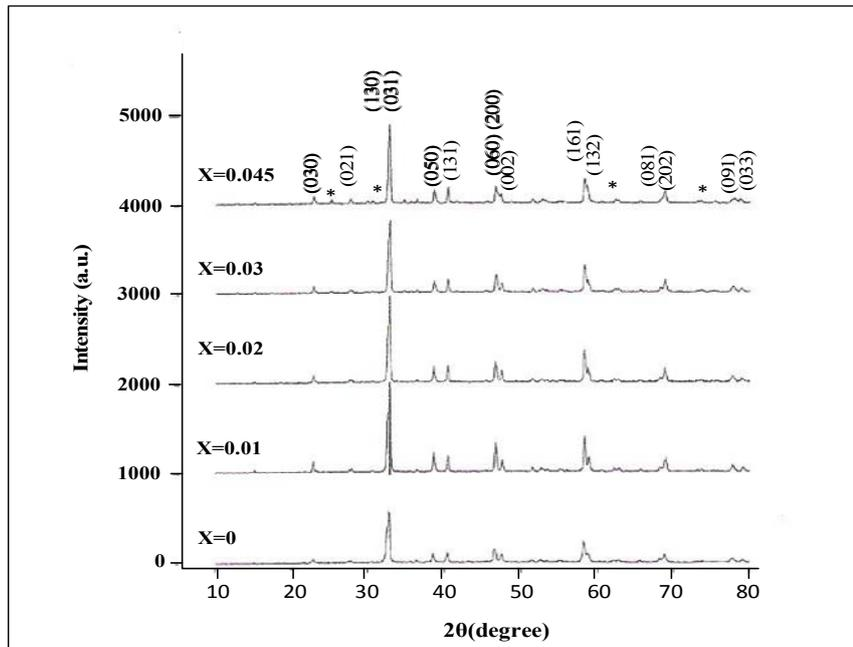
Figure 1: X-ray diffraction patterns for components  $YBa_2Cu_{3-x}Al_xO_{6.5+\delta}$ .
