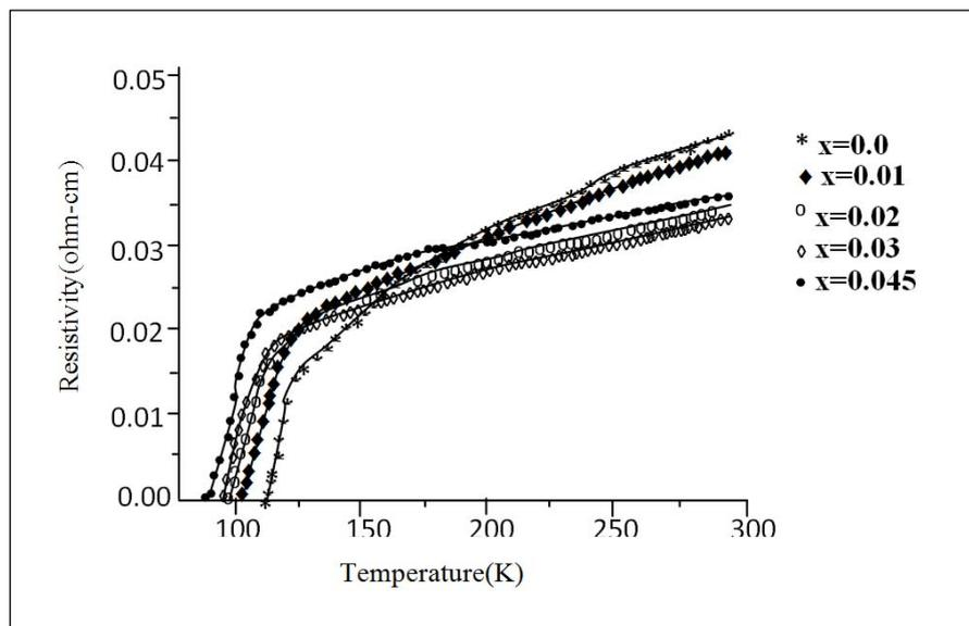
Figure 2: Resistivity versus temperature for  $YBa_2Cu_{3-x}Al_xO_{6.5+\delta}$  compositions.
