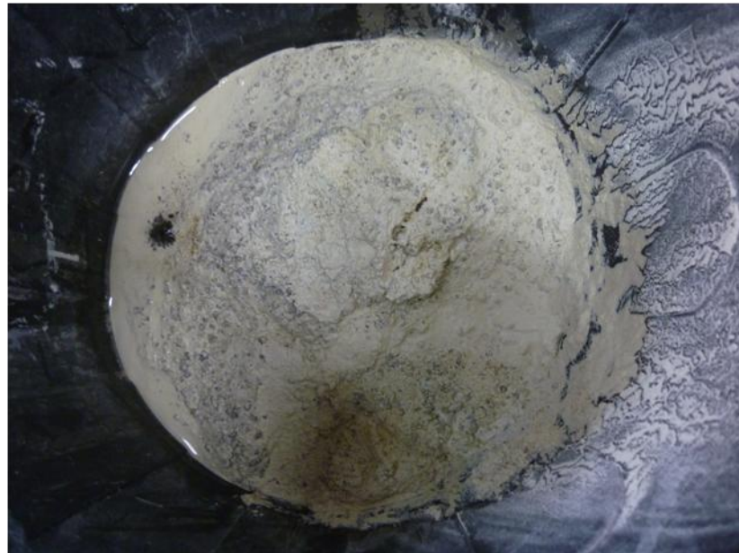
Figure 3.16 The samples fully destroyed after submerged in water for ten minutes.
