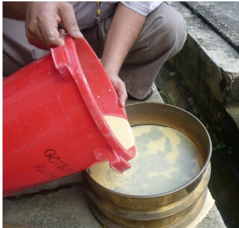
Figure 3.19 Starting the wet sieving by using sieve size 425 \mu\text{m} set over sieve size 63 \mu\text{m} .
