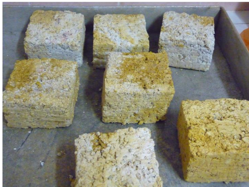
Figure 3.36 Step 6: Collect the sample carefully and put it on sealed plastic to keep the natural moisture content (procedure to preparation samples for the direct shear test).
