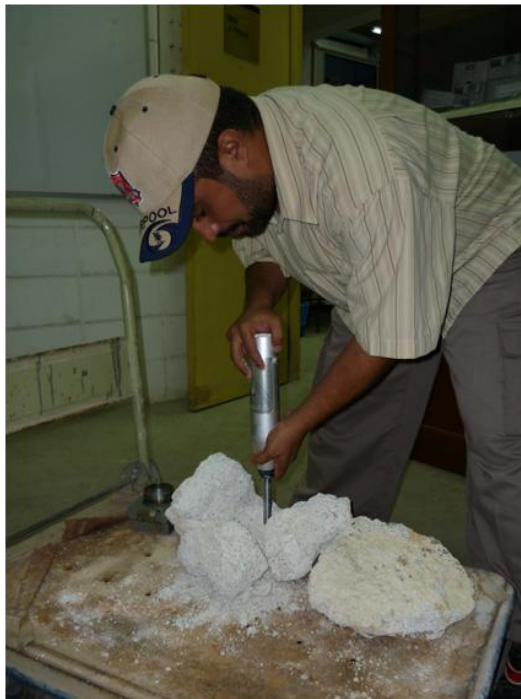
Figure 3.8 Measuring surface of hardness by Schmidt (rebound) hammer test at the laboratory.
