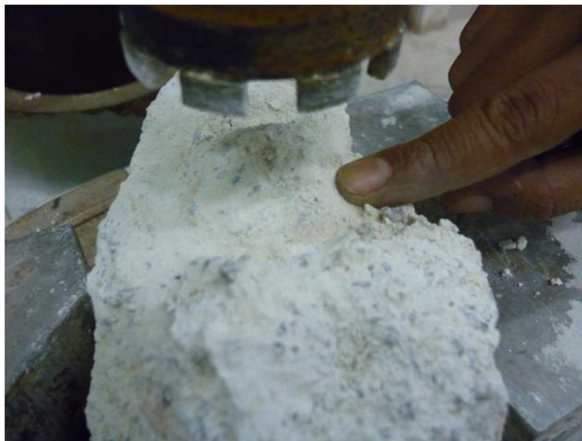
Figure 3.25 The dry sample was disturbed partially during use coring apparatus to prepare it for the direct shear test.
