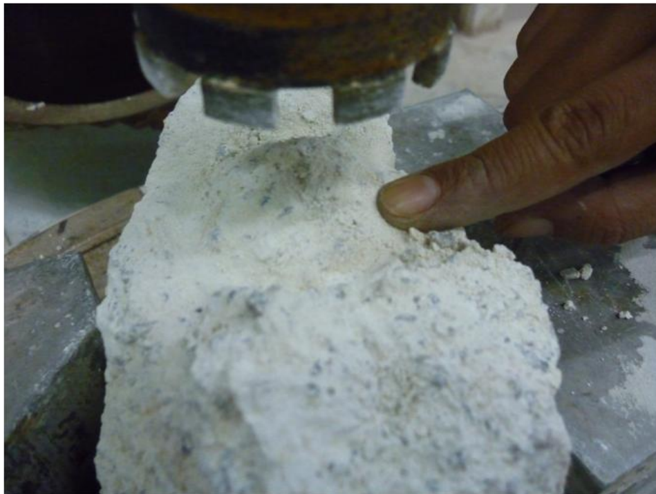
Figure 4.8 The sample was destroyed during coring to prepared regular sample (cylindrical i.e. core sample ) for point-load test PLT.
