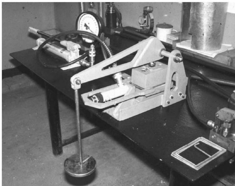
Figure 3.24 Shear machine of the type used for measurement of the shear strength of sheet joints in Hong Kong granite (Evert Hoek, 2000).
