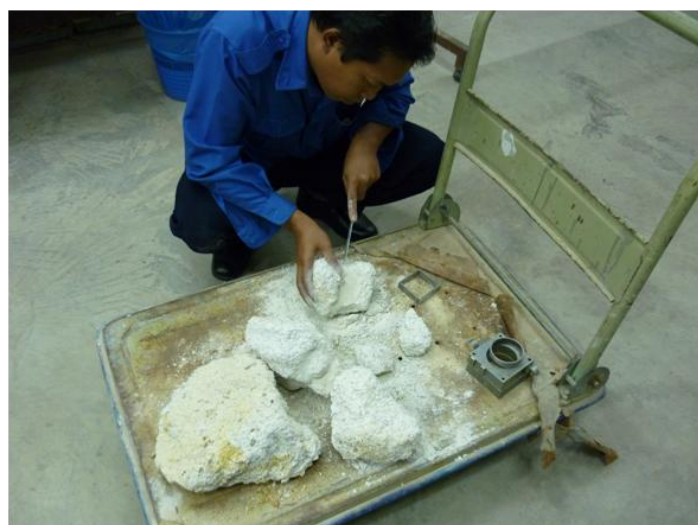
Figure 3.11 Preparation the irregular shape samples for point-load test.
