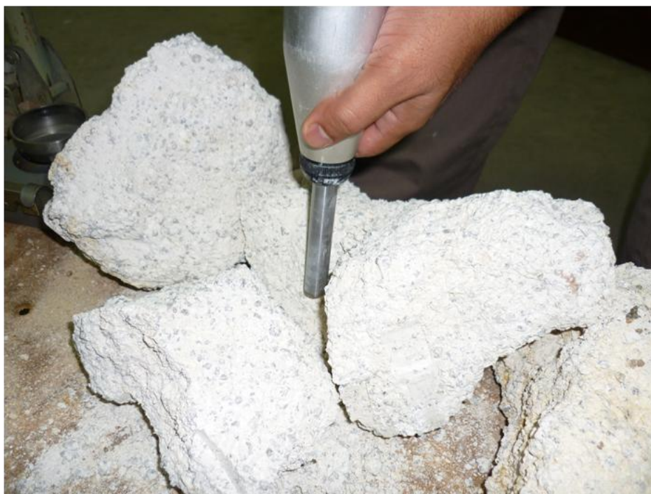
Figure 4.7 The sample was destroyed during the Schmidt (rebound) hammer test.
