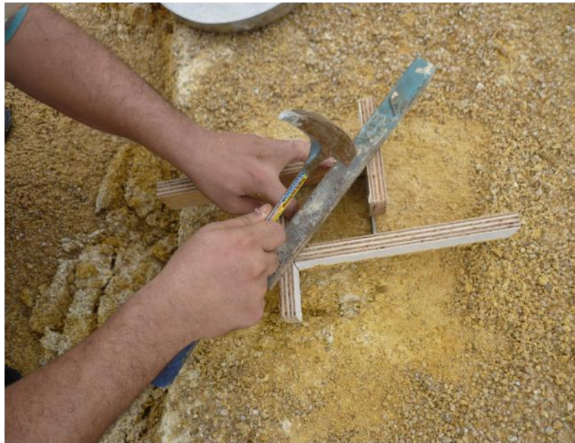
Figure 3.33 Step 4: Use the fabricated wood to penetrate more (procedure to preparation samples for the direct shear test).
