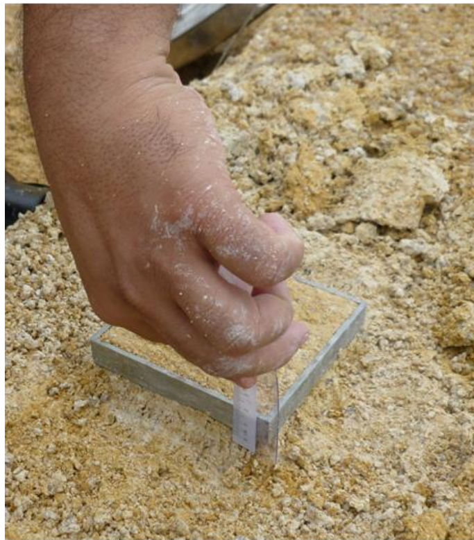
Figure 3.34 Step 5.a: Measuring the sample thickness (procedure to preparation samples for the direct shear test).
