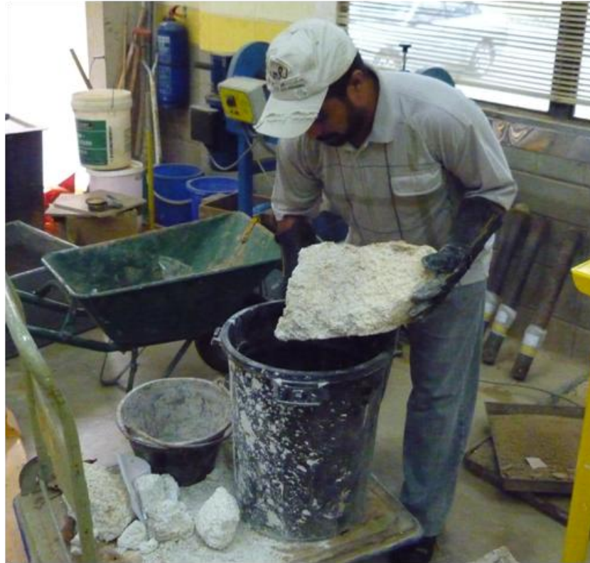
Figure 3.15 Submerging the sample into water.
