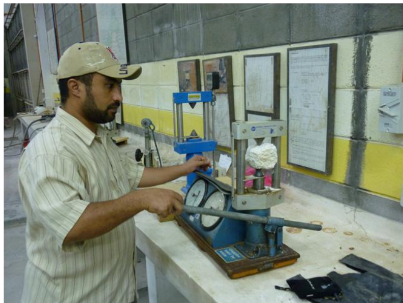
Figure 3.13. Applied the pressure over the irregular sample by the point-load apparatus.
