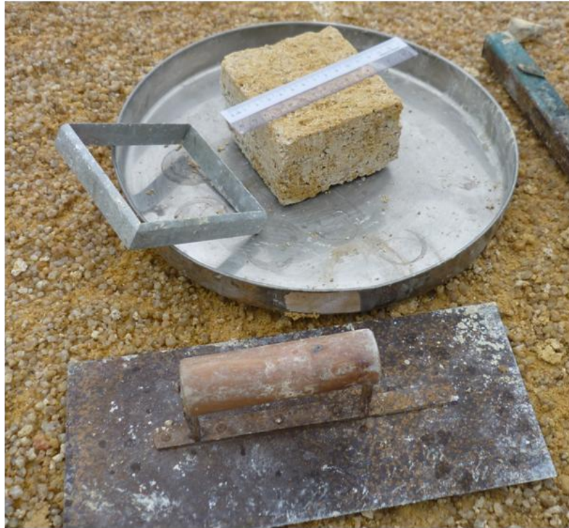
Figure 3.35 Step 5.b: Extract the sample by using the metal sheet, when the thickness of sample enough (procedure to preparation samples for the direct shear test).
