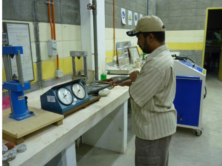
Figure 3.12 Preparation the point-load apparatus.
