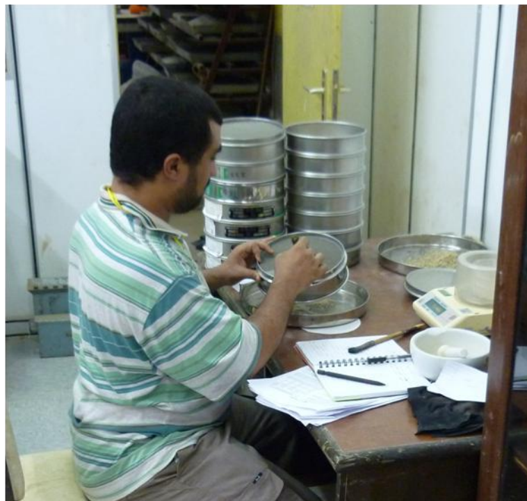
Figure 3.21 Brushed the dry particles during carried out the last stage of wet sieving.
