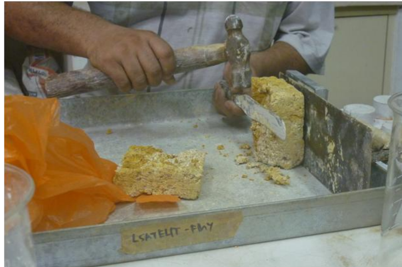
Figure 3.37 Step 7: Reshape the sample when it still wet in order reduce the thickness (procedure to preparation samples for the direct shear test).
