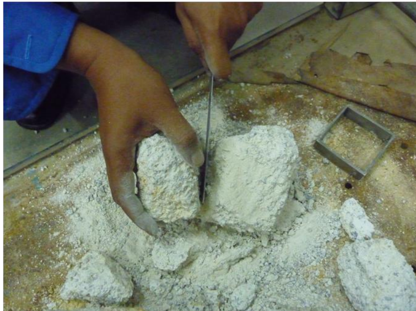
Figure 3.27 Preparation of sample by cutting for direct shear test.
