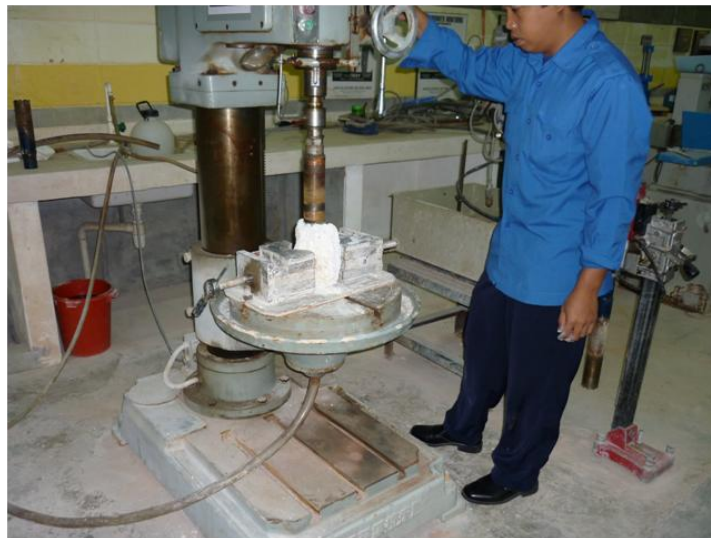
Figure 3.10 Preparation the core samples for point-load test.
