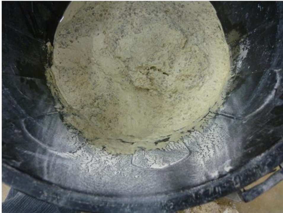
Figure 4.10 The samples fully destroyed after submerged in water for ten minutes.
