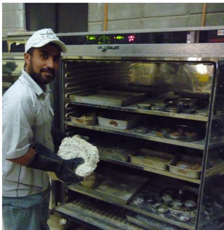
Figure 3.7 First step to prepare the dry samples by placed the samples into the oven.
