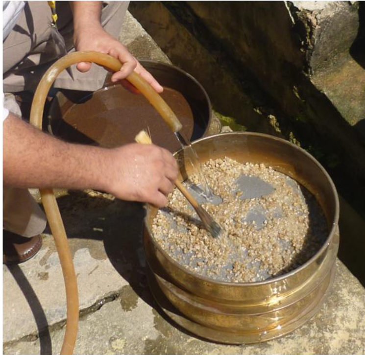
Figure 3.20. Brushed and washing the wet particles during carried out the wet sieving.
