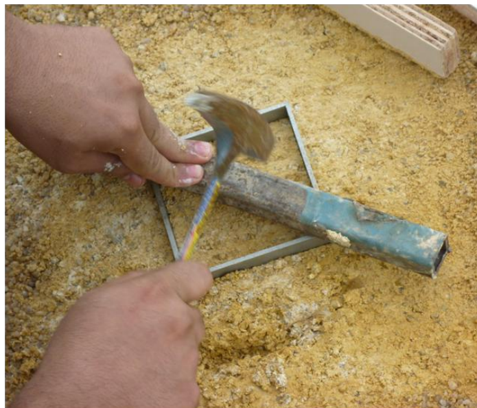
Figure 3.30 Step 2: Put the cutting ring then the metal rod over it and starting puncture by hammer (procedure to preparation samples for the direct shear test).
