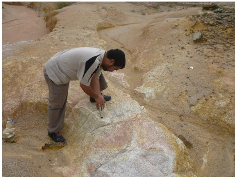
Figure 3.6 Measuring surface of hardness of older alluvium by Schmidt (rebound) hammer.
