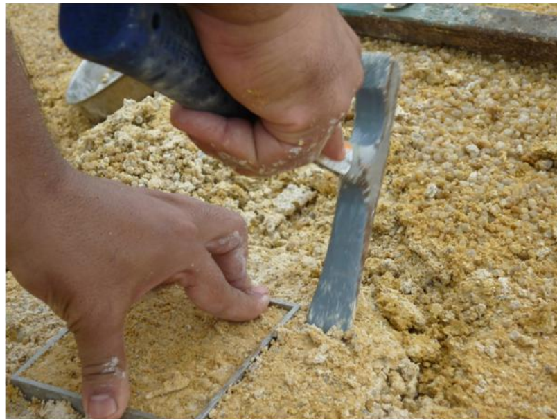
Figure 3.32 Step 3.b: Material surrounding cutting were cleared to retrieve samples (procedure to preparation samples for the direct shear test).
