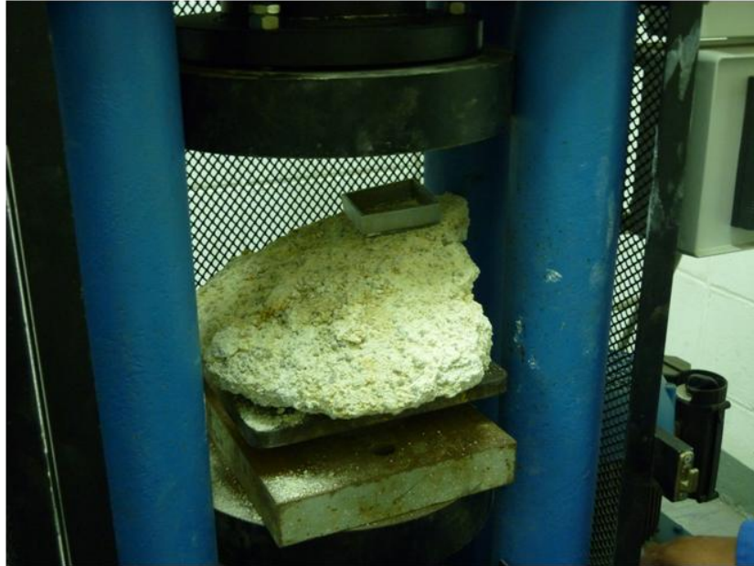
Figure 3.26 Photo shows on effort to prepare cubic sample for direct shear test by pressure with hydraulic machine (the sample was broken).
