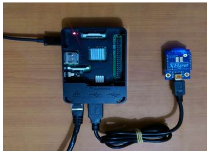
Figure 5. Hardware implementation of the main station node
