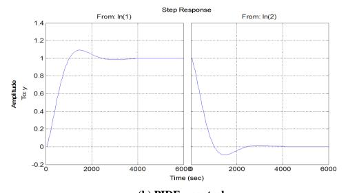
(b) PIDF – control Fig.(10) Response to set point ysp and disturbance (d).
