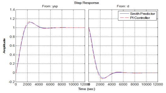
Fig. (11b) Control response to step input comparison between PI- Control and Smith predictor.
