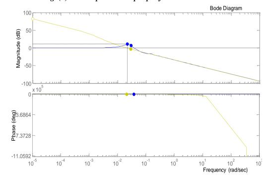
Fig. (6) Bode plots for PI- control system.
