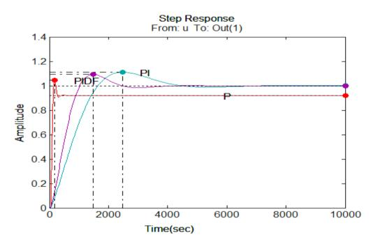
Fig. (11) Comparison between P,PI, PIDF Control response to step input.
