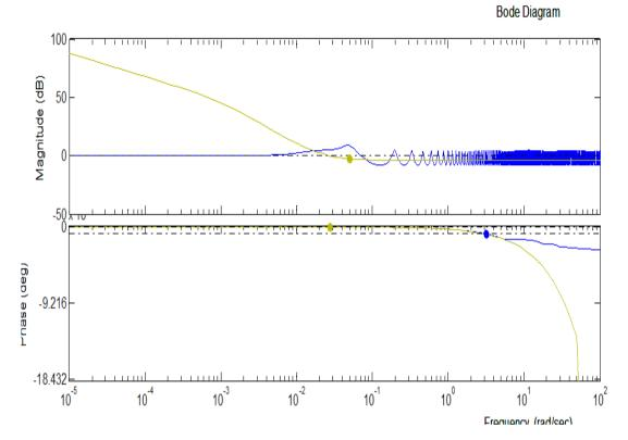
Fig. (7) Bode plots for P- control system.
