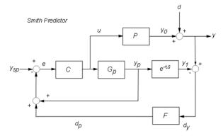
Fig. (1) Signal flow diagram of a Smith-Predictor.
