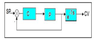
Fig. (2) Equivalent transformation of the Smith predictor scheme [9].
