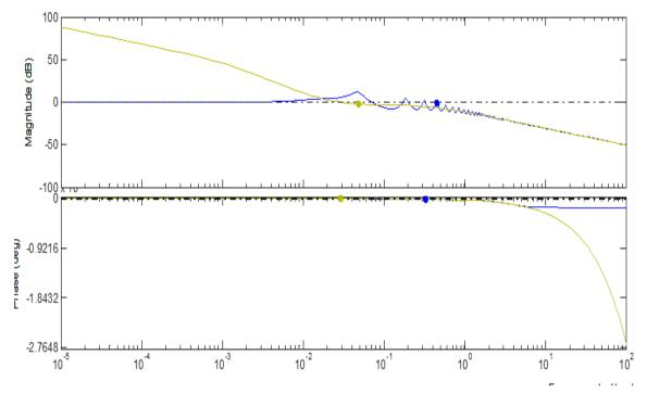
Fig. (9) Bode plots for PIDF- control system.
