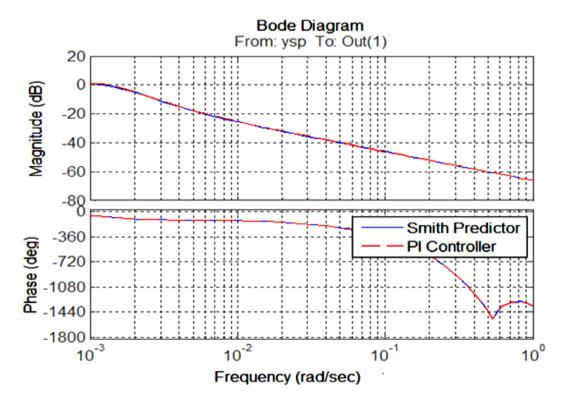
Fig. (11a) Bode plots comparison between PI- Control and Smith predictor.
