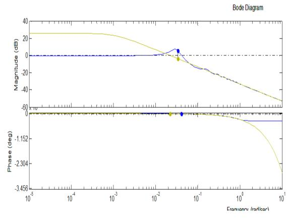
Fig. (8) Bode plots for PID- control system.
