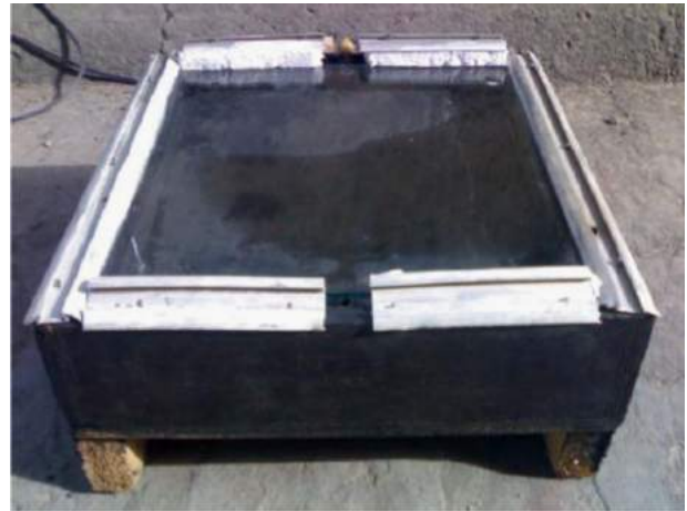
Fig. 31. Direct absorption solar collector (Verma and Kundan [94]).
