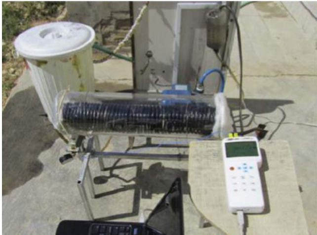
Fig. 47. Cylindrical solar collector and the experimental setup (Goudarzi et al. [136]).
