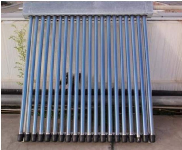
Fig. 3. Photograph of the heat pipe solar collector (Du et al. [42]).
