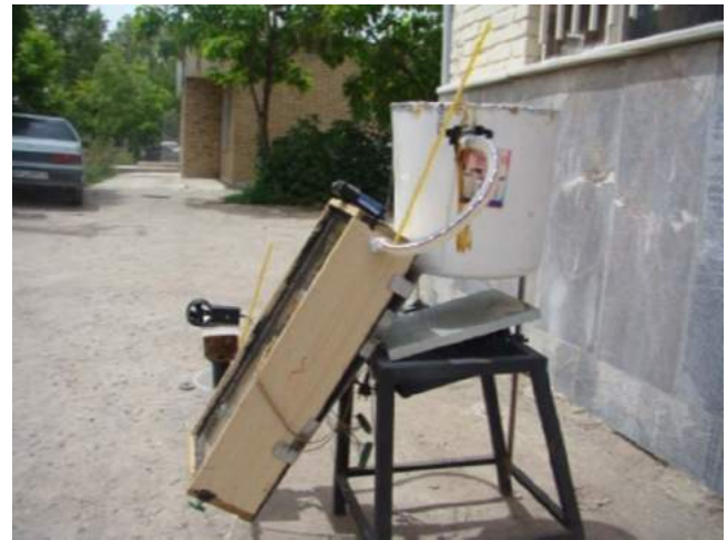
Fig. 15. The experimental flat plate solar collector (Chaji et al. [63]).
