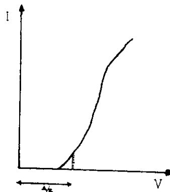
Fig. 2. I-V characteristic for SIN junction
