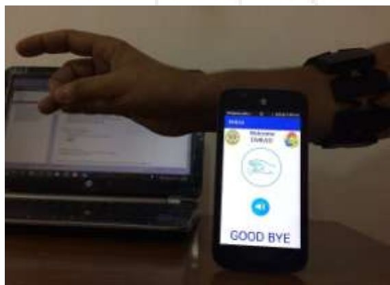
Figure 10: The Gesture “DoubleTap” with its Related phrase “GOOD BYE” “on the Smartphone Screen.
