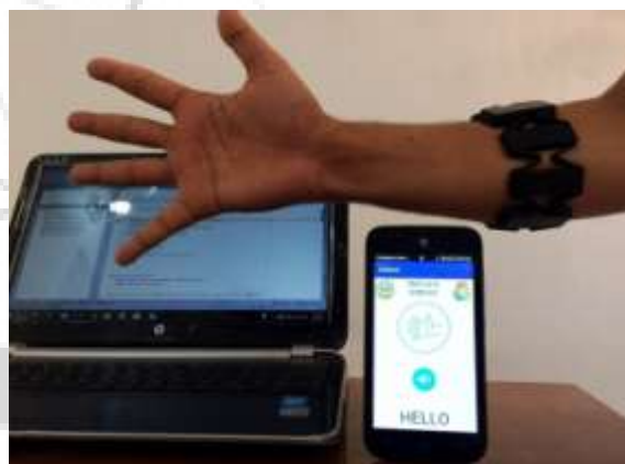
Figure 6: The Gesture "Fingers Spread" with its Related Word "HELLO" on the Smartphone Screen.
