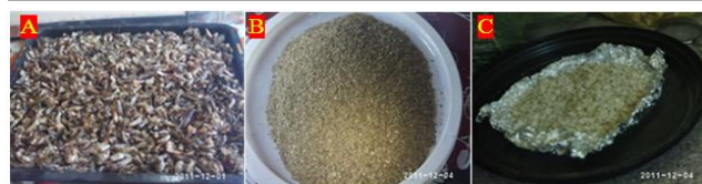
Fig.1 picture of chitosan production from shrimp shell , (A) shrimp shell , (B)chitin , (C) chitosan
