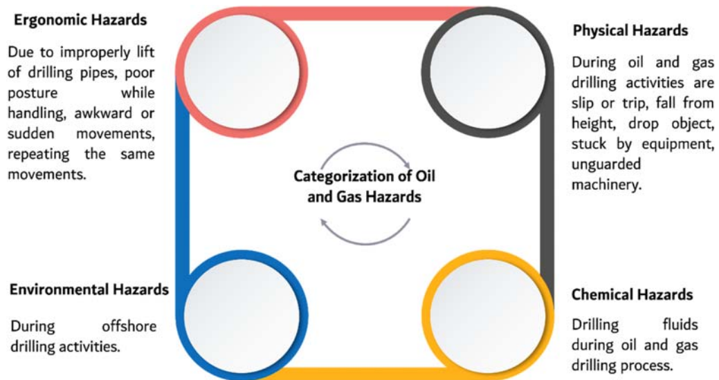
Figure 9.1 Oil and gas hazards categorization.
