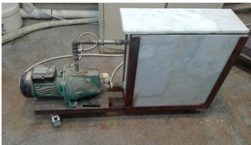
Fig. 3: Erosion-corrosion apparatus depend on (G73) ASTM. This device designed during the study
