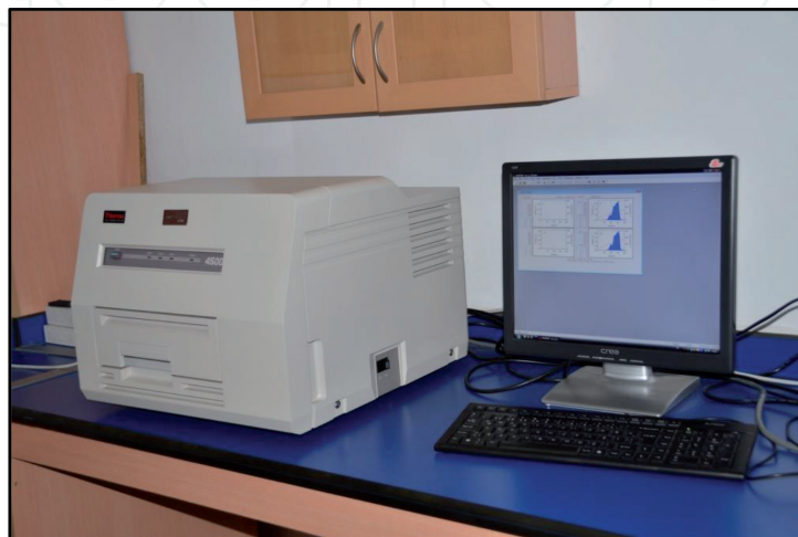
Figure 4. THERMO SCIENTIFIC 4500 TLD READER [25].
