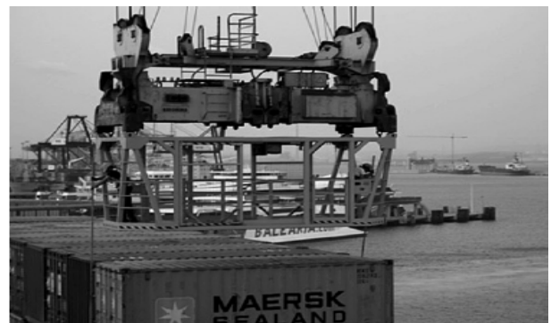
Figure 1. Detail of stevedore unlashng containers at height from a safety cage
