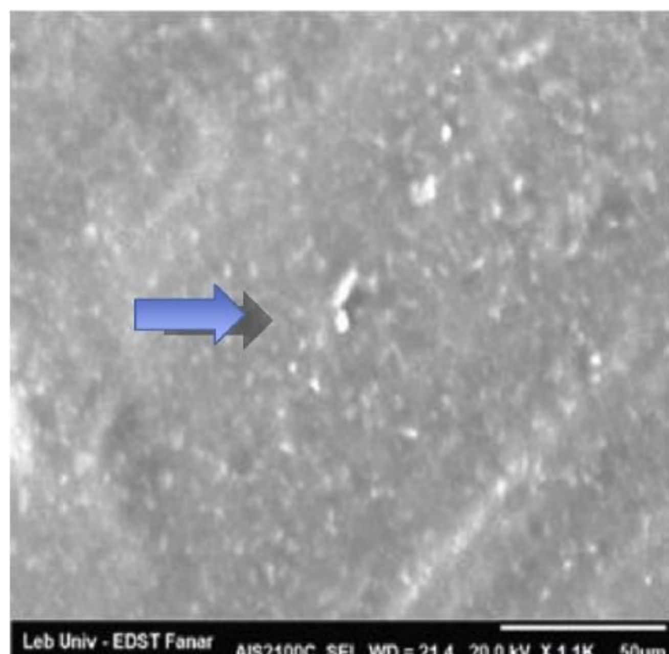
Fig. 6. SEM micrograph of IPS Empress Direct replica one-year after bleaching (1000x magnification).
