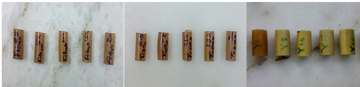
Figure 2 Compression test samples of epoxy composites with different reinforcements Fiber glass, (b) TiO 2 , (c) Y 2 O 3 and different volume fraction.
