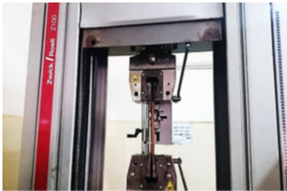
Figure 4 universal testing machine (Zwick / Roell Z100)
