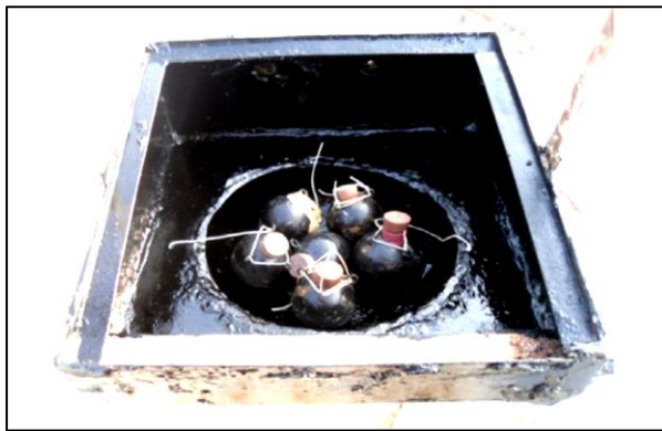
Fig.5: Solar still absorber with 6 PCM balls[24]
