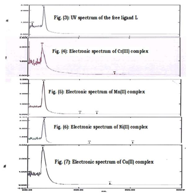
**Figs. (3-7):** Electronic spectra of the Schiff base and its complexes
