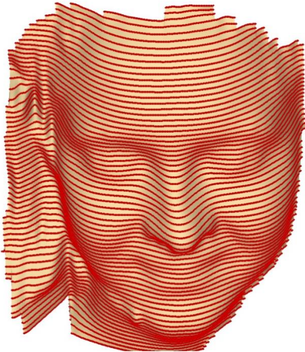
Figure 5: On the mesh, an estimated point is used to indicate the points where each horizontal and vertical plane intersects with the other. 39,743 valid intersection or vertices can be found in the model displayed.
