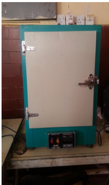
Figuer(3.3): laboratory oven (lab-tech), volt 230, watts 500 Serial No: 14125, size: 14x14, Manufacturing in India
