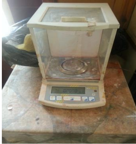
Figuer (3.1) KERN electronic balance Capacity 120 g Readbility:0.1m
