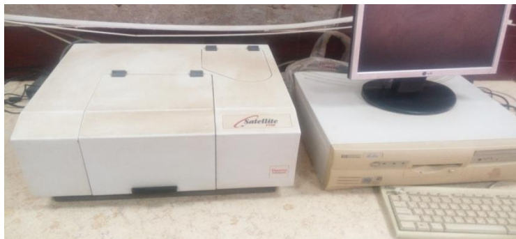
Figure (3.7)... Satellite FTIR ... Serial N0 20010102 Voltage. +5/+15/-15 VDC... Manufactured in U.S.A
