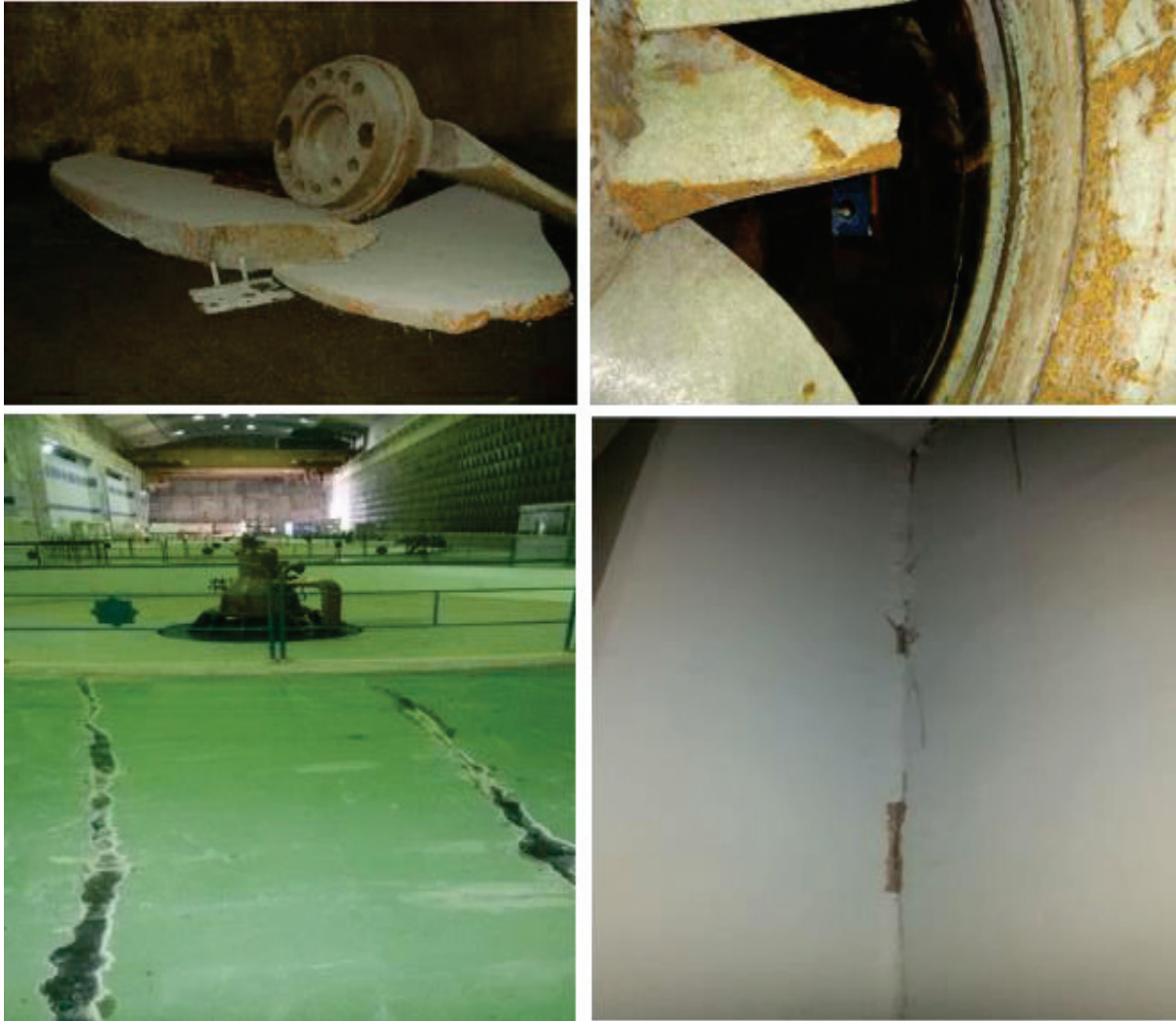
FIGURE 2. Runner blade damage (top row), and structural cracks in Haditha plant (bottom row). Image courtesy of Ministry of Electricity/Iraq.
