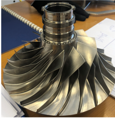
Figure 2: High pressure compressor
