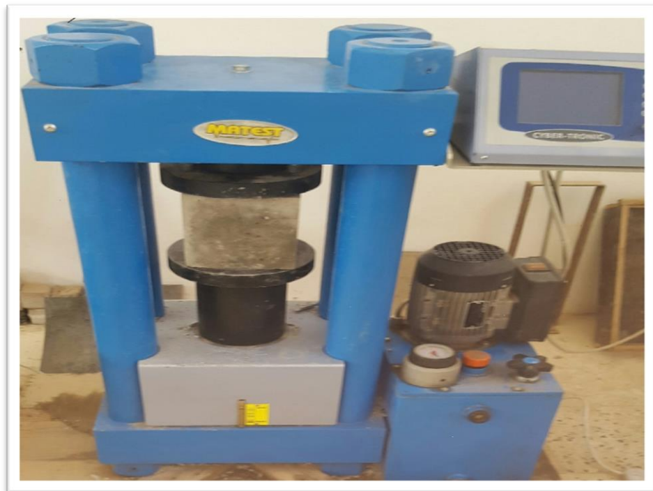
Figure 2: Cube inside Compressive Strength Machine
