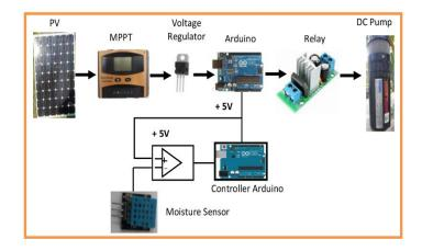
Figure 1. Block diagram of irrigation system
