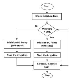
Figure 3. Irrigation procedures flowchart
