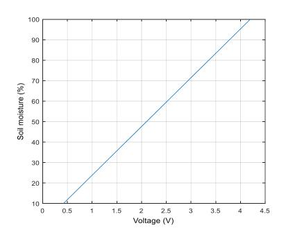
Figure 5. Voltage sensor V soil (%) moisture
